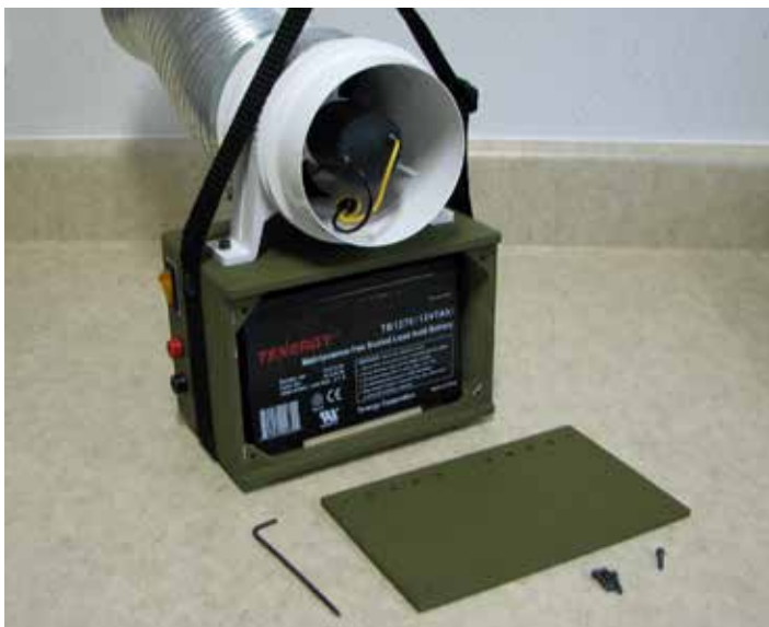
View of Cooling Fan showing access to battery.
