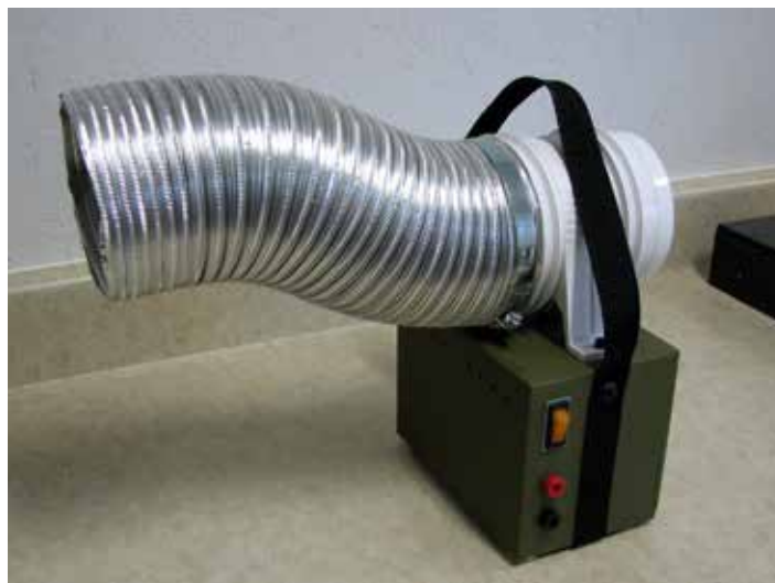
View of Cooling Fan showing switch and charge jacks.
